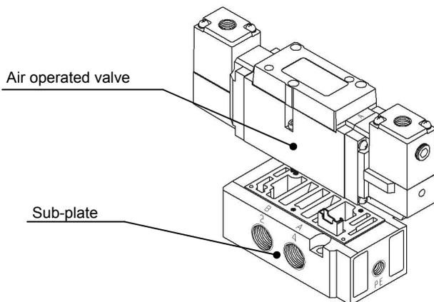
Tightening torque for mounting bolt : 2.8N·m
