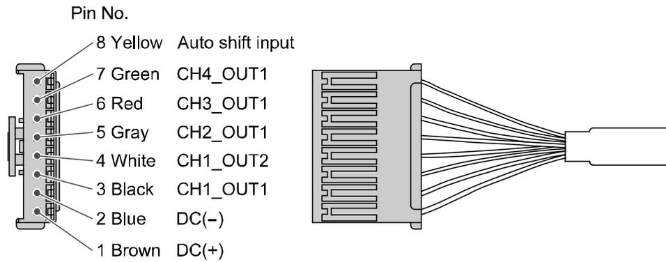
■ Internal circuit and wiring example
