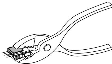
\*: The connector cannot be re-used once it has been fully crimped.
