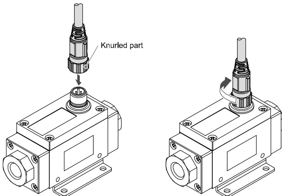
**Attaching the sensor connector to the lead wire (When the product connects to the PF2A2□□)**
