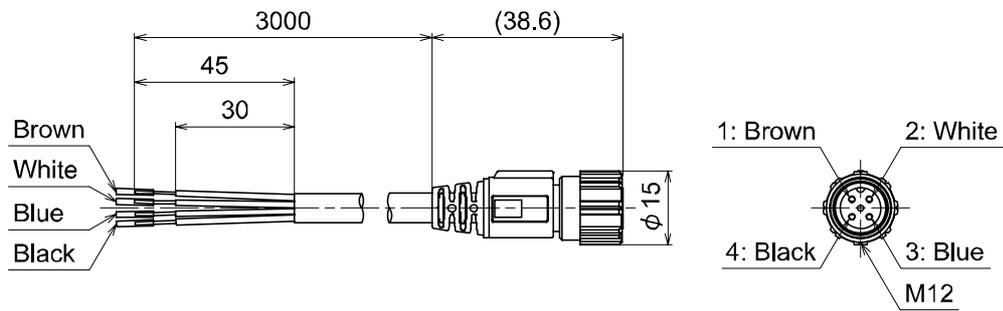
Lead wire and connector (Angle): ZS-37-B
