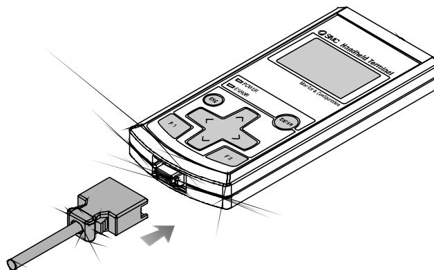
•Connect the M12 connector on the Handheld Terminal cable into the connector (PCI) of the SI unit.
