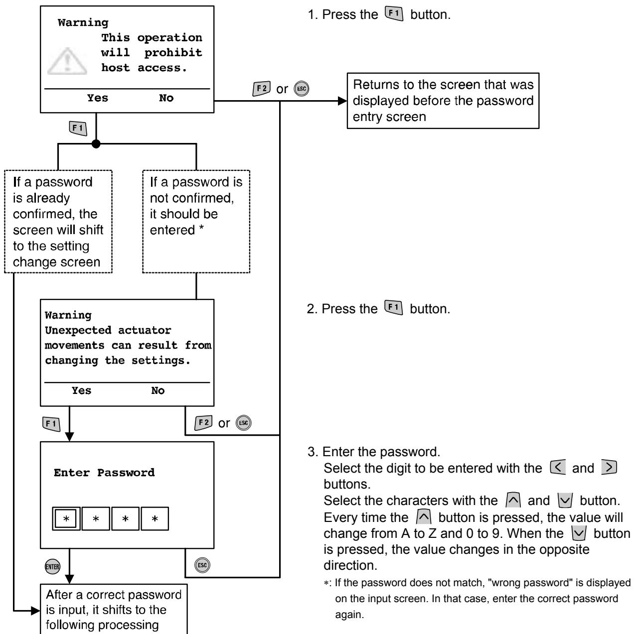
\*: When changing the settings after the unit has recovered from the POWER SAVE mode, it is necessary to enter the password again.
