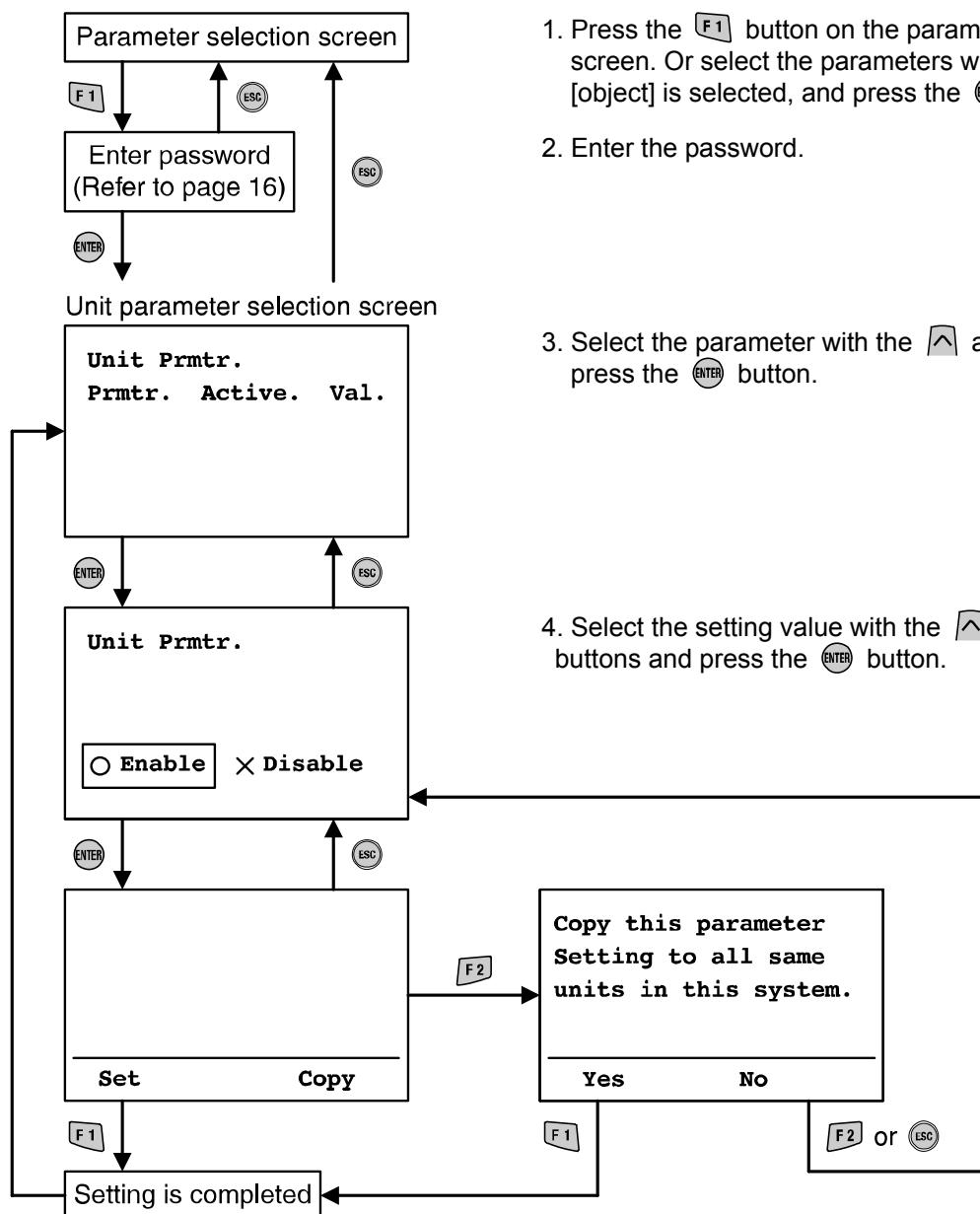
1. Press the **F1** button on the parameter selection screen. Or select the parameters where the [unit] in the [object] is selected, and press the **ENTER** button.
