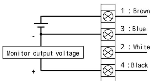
Only use equipment with a minimum load impedance of 100k .
