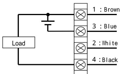
When a current of approx. 150mADC or more is applied, the over current circuit is archived, “Er.5” is displayed and the operation stops. Please use with installing the load that the output current becomes to 80mADC or less.
