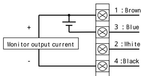
Only use equipment with a maximum load impedance of 250 .
