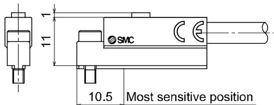
\*: Mounting the white heat shrinking tube with only D-P3DWSE.
